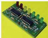
A must for photographers and computer users. Use it in your motor home to monitor the AC generator. The AC voltage is indicated in 6v steps by seven multi-colored LEDs.
