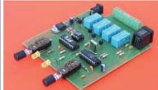
Now you can control 4 separate devices with DTMF tones from anywhere in the world using your telephone! Simply connect your Phone Tone Genie to your phone line and program in a security
