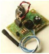
Use this kit to control cooling fans. It senses heat and turns on a fan. The fan can be a ceiling fan or a fan in your computer, anything that needs cooled. Output is 100mA.
