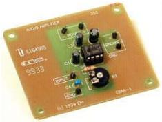
This kit teaches how amplifiers take a small signal and "magnify" it to drive a small speaker or headphone. It's based on the LM386 Low Voltage Power amplifier.
