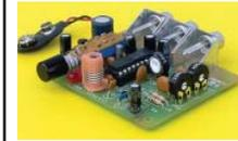
Have your own FM radio station. Any stereo signal you plug into the FMST-100 transmitter kit will be transmitted to any FM radio tuneable from 76 to 108MHz FM. Plug in your CD player, tape deck and have a
