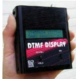
Press a button and learn every number dialed on your phone while you were away! **Stores the last 490 digits it receives. Connects to a phone, scanner, amateur radio, or etc. Decodes any DTMF signal transmitted.**
