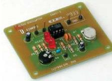
Sine waves are "pure" audio tones typically used to test audio equipment. This audio oscillator kit produces sine wave audio signals. Output amplitude is adjustable. Use this kit to learn
