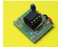
This easy to build kit will give you the dots and dashes for practicing the Morse Code. You can use this as a signal tracer to repair audio amplifiers. Power requirement 6 to 15 volts DC.
