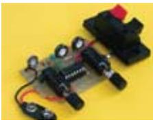
This is the kit everyone has been asking for. Turn your digital volt ohm meter into an inductance meter. It will read inductors 3uH to 7MH. Power requirement 9v DC. SIZE: 1.75" x 2.5"
