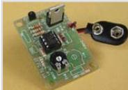
Don't ever get stuck with a flooded basement or over fill your water bucket. When the liquid level reaches the sensor it automatically turns the pump on or off. The Water Alarm supplies you with 80 mA of
