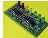
If battery status is important, you need this kit. This kit uses 7 LEDs to monitor 12v DC in 1v, 1/2v, or 1/4v steps. Monitor 8v or 5v in 1/4v steps. Great for boats, motor homes, model planes or race car ni-cads. All parts and instructions are included.
