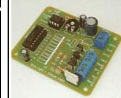
Use this kit like a theatre marquee. Every forth LED chases around the display to give you a dazzling effect. You can use up to 40 LED's. Only your imagination limits the possibilities. We supply 16 RED LED's. PC Board size: 2.25" x 2.75" Power Requirement: 7.5 to 15 VDC
