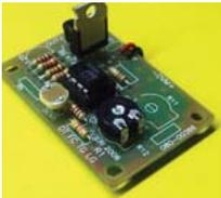
Turn anything on or off with light. Turns on at night off at daylight automatically. As the light touches or leaves the sensor it delivers 80mA of output to run a relay.
