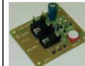
These power supplies will supply DV voltage of the proper magnitude and type for most kits, and supplies a well regulated and filtered +5vDC, and a variable output from +6 to +10vDC. and has thermal overload protection,
