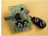
The DT-3 kit will turn your digital volt ohm meter into an accurate digital thermometer with .1 degree resolution. Measure temperatures from -40° to 250F°. The remote sensor is .25" sq. and can be
