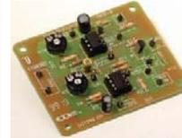
Based on the LM555 Timer Chip, a highly stable device for generating accurate time delays or oscillation. When a switch is turned on or off, mechanical
